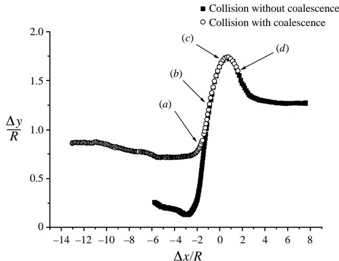
FIGURE 13. Plot of  $\Delta y/R$  vs.  $\Delta x/R$  for  $Ca = 0.13$ ,  $\lambda = 0.36$ . The circles ( $\circ$ ) correspond to the collision with coalescence of figure 12. The squares ( $\blacksquare$ ) correspond to a collision between two drops generated by break-up of the drop formed upon the coalescence shown in figure 12.
