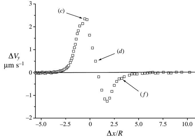
FIGURE 11. Plot of the relative velocity  $\Delta V_y$  between the drops in the  $y$ -direction *vs.*  $\Delta x/R$ , same experiment as in figure 5.
