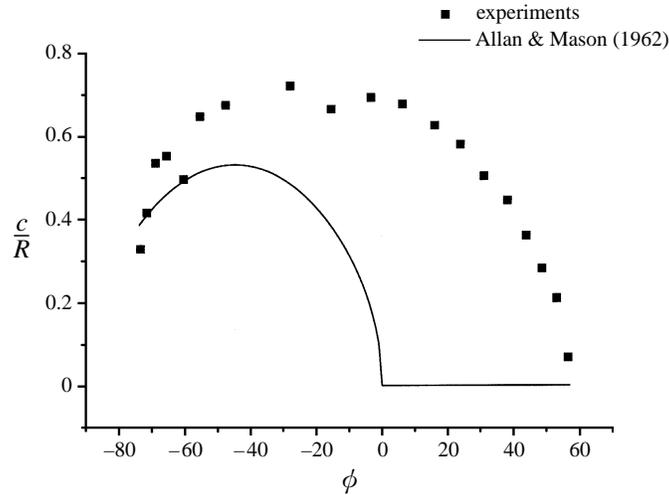
FIGURE 16. Plot of  $c/R$ , where  $c$  is the extent of the near-contact region, as a function of  $\phi$ . The squares are experimental data; the continuous line corresponds to the Allan & Mason model (1962).
