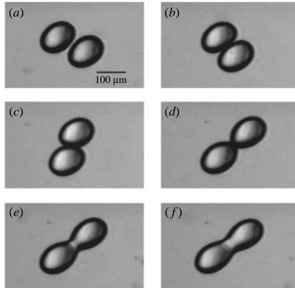
FIGURE 12. Sequence of images showing a collision with coalescence.  $Ca = 0.13$ ,  $\lambda = 0.36$ .
