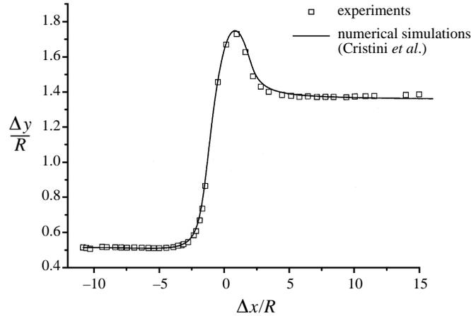
FIGURE 17. Comparison between experiments and numerical simulations by Cristini *et al.* (unpublished work). The open squares are experimental data of  $\Delta y/R$  vs.  $\Delta x/R$ , the continuous line is the numerical simulation.  $Ca = 0.135$ ,  $\lambda = 1.37$ .
