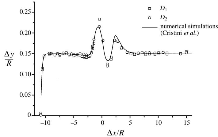
FIGURE 18. Comparison between experimental and numerical values of the deformation parameter  $D$  vs.  $\Delta x/R$ . The squares and the circles correspond to the deformation parameters  $D_1$  and  $D_2$  of the two drops, the continuous line is the numerical simulation (Cristini *et al.* unpublished work). Same conditions as in figure 17.
