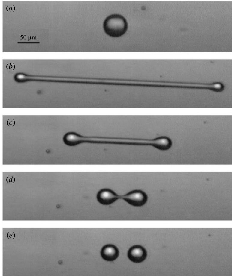
FIGURE 2. Break-up of a sheared drop after stopping the flow. (a) Drop at rest; (b) drop extended by shear; (c) and (d) drop retraction after stopping the flow; (e) the two drops generated by break-up.
