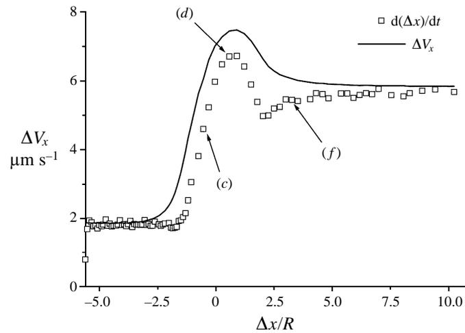
FIGURE 10. Plot of the relative velocity  $\Delta V_x$  between the drops in the  $x$ -direction *vs.*  $\Delta x/R$ , same experiment as in figure 5. The continuous line has been calculated as  $\dot{\gamma}\Delta y$ .
