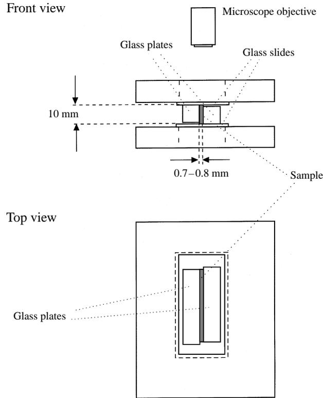
FIGURE 1. Schematic of parallel plates assembly.
