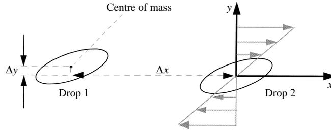
FIGURE 4. Frame of reference used to represent collision data.
