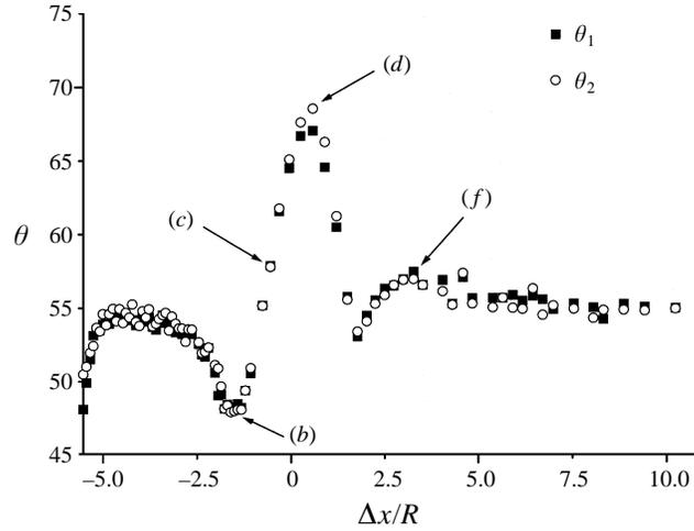
FIGURE 9. Plot of the angle  $\theta$  between drop major axis and velocity gradient direction *vs.*  $\Delta x/R$ , same experiment as in figure 5.
