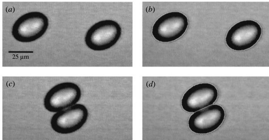
FIGURE 3. (a) Digital image of two drops during approach; (b) same image as in (a), drop contours as identified by image analysis are shown in white; (c) image of two colliding drops in close contact; (d) same image as in (c), the contours of the two drops have been separated and are drawn as white lines.  $Ca = 0.13$ ,  $\lambda = 1.4$ ,  $R = 17 \mu\text{m}$ .
